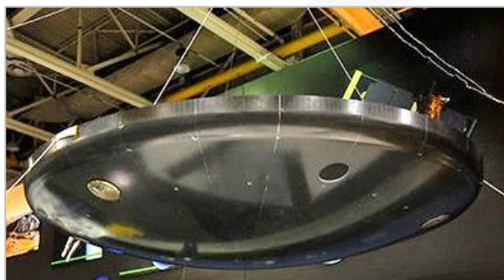
Carbon Laminate Skin (EFT1 Shown)
