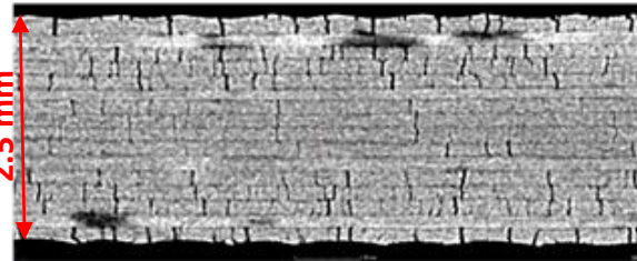
X-ray CT data of microcrack damage
