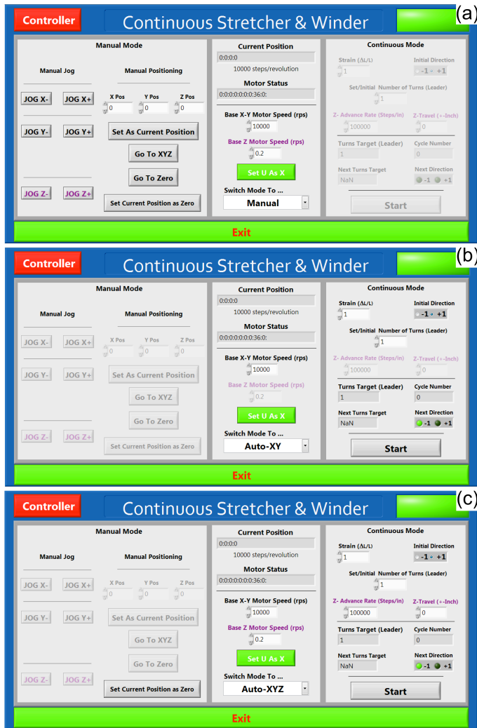
Figure 3. Screenshots from the user interface of CSAW, a LabVIEW based tool developed for controlling a continuous tape stretcher and winder showing options available under (a) the "Manual" (initial setup), (b) "Auto-XY" (stretching) and (c) "Auto-XYZ" (winding) modes.
