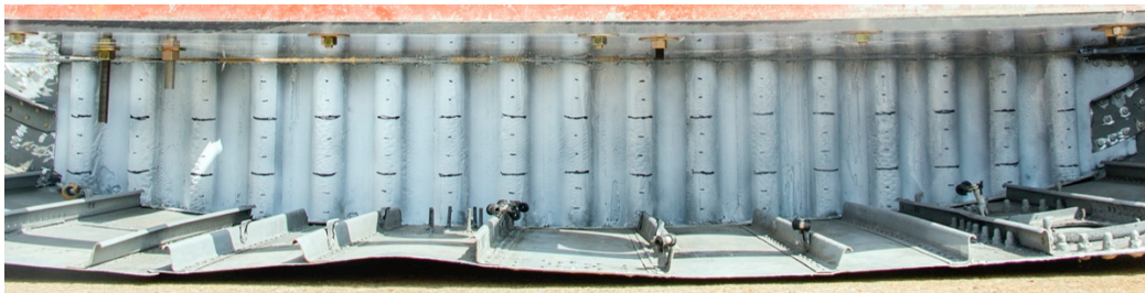
Figure 10. Pre-test photograph of the sinusoid energy absorber, as retrofitted into the barrel section.
