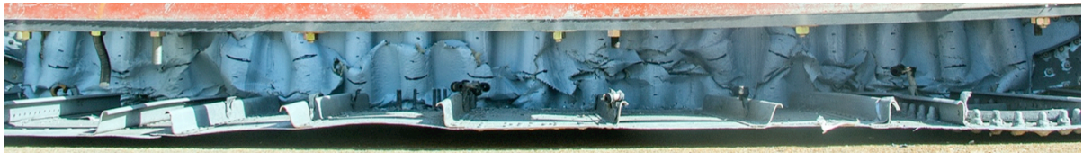
(b) Post-test photograph highlighting the post-test crush response of the sinusoid.
