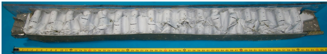
Figure 18. Photograph of the sinusoid foam sandwich energy absorber, removed from the test article. Note that the subfloor section is lying on its side with a portion of the polycarbonate floor still attached.
