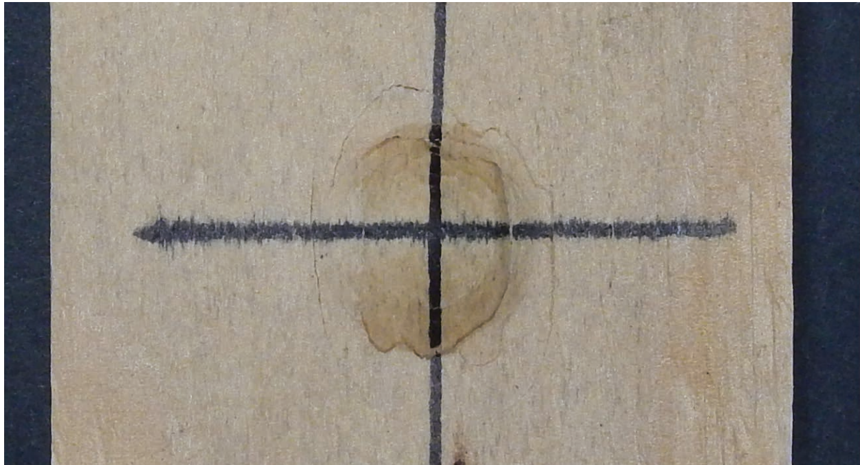
Figure 13. Wood impact sample from 5-lb weight impact test.
