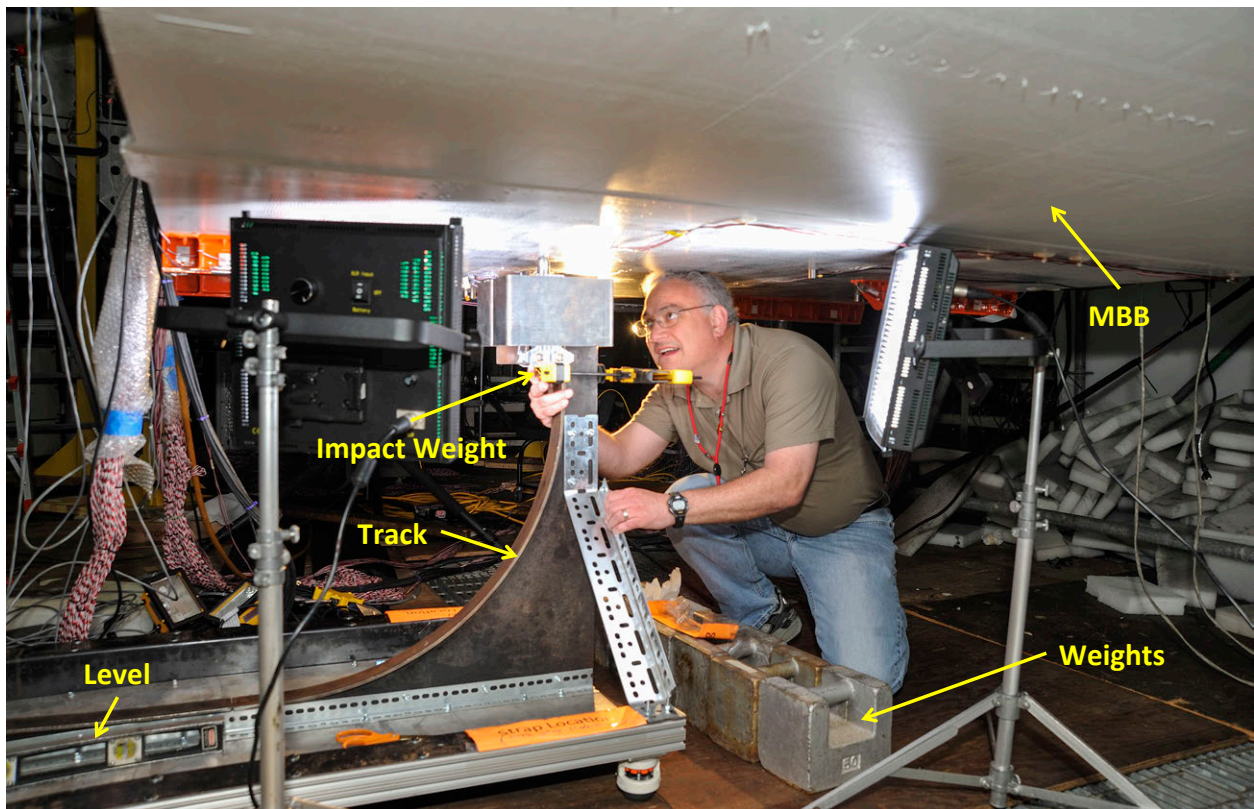
Figure 15. Alignment of impactor for exterior skin impact.
