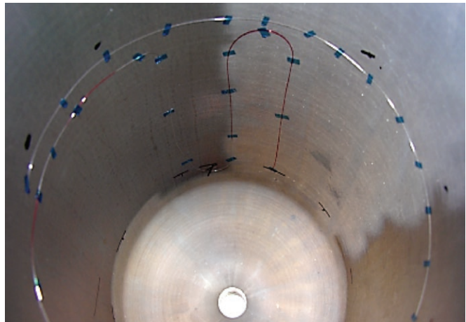
Internal strain monitoring within a composite tank
