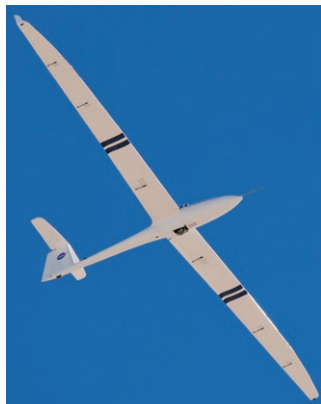
This unmanned sailplane shows off its graceful high-aspect-ratio wings.
