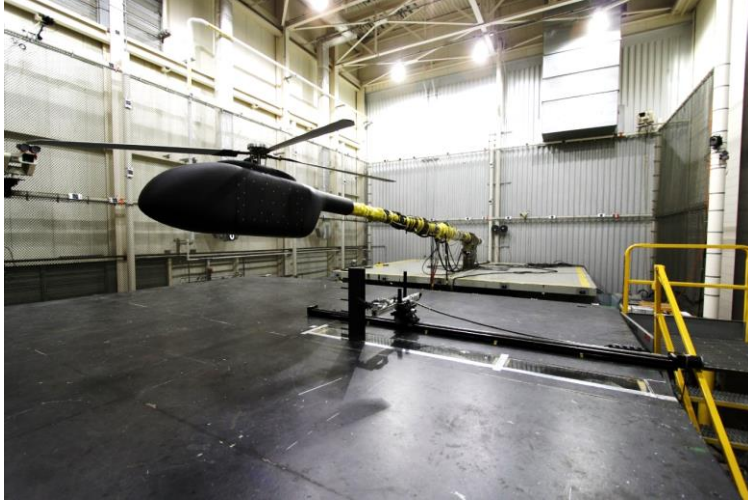
Figure 4. GRMS with ROBIN-Mod7 installed in RTC during T613.
