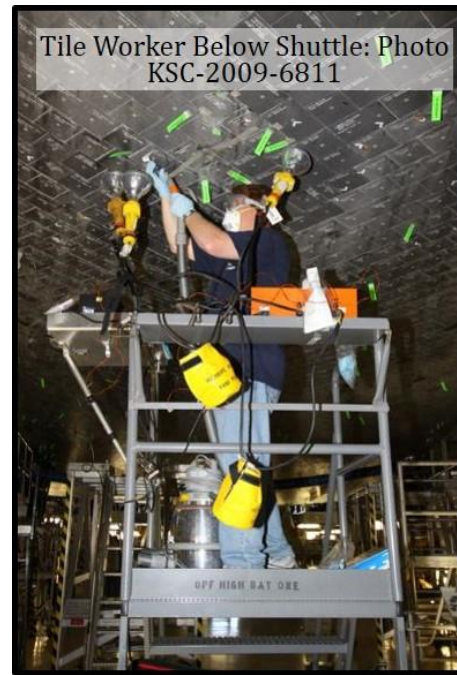
Figure 10: Work Stands with Attachments can Place Personnel/Tools/Equipment at Arm's Reach
