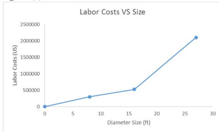
Figure 7(b). Effect of tank barrel diameter on total cost vs. size.
