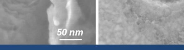
□ 900-1000 °C/10h: larger sizes; through-thickness □ Rough edges due to oxidized boron build-up can be removed by nitric acid treatment for defined shapes
