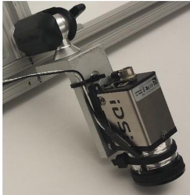
Figure 9. Camera with Lens Heater Installed
