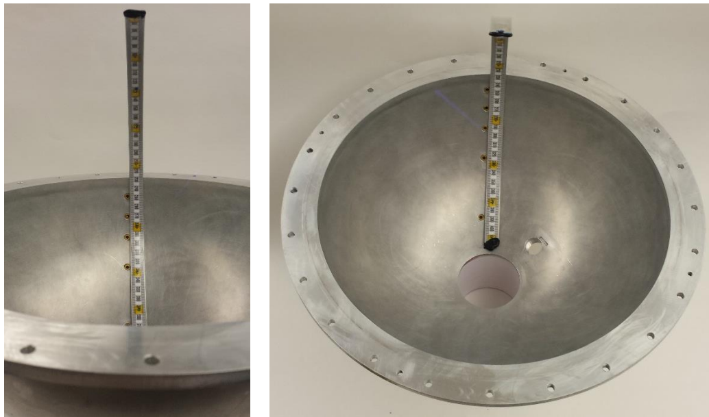
Figure 12. Final Fluid Sensor Installed in Tank
