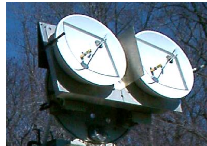
Quinstar 24" Cassegrain Antennas simplified to a small horn during flights
