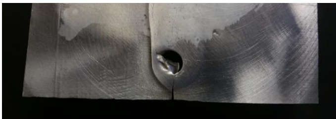
Figure 18. Root side image of the gap in a 3.18 cm thickness weld panel in advance of the weld tool at the end of the weld.
