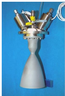
Figure 7. Aerojet 100-lb f LOX/LCH 4 RCE
