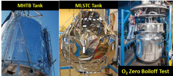
Figure 20. a. Multipurpose Hydrogen Test Bed (MHTB) tank (left) and b. Methane Lunar Surface Thermal Control (MLSTC) tank (center) and c. LOX zero-boiloff test (right).
