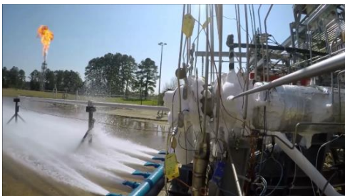
Figure 19. Additively Manufactured LOX/LCH 4 Turbo-pump Testing
