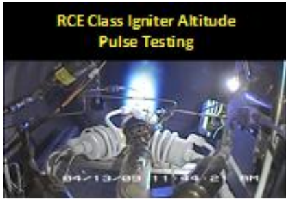
Figure 2. RCE Class spark torch igniter (Firing)
