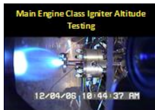
Figure 1. Main Engine Class Spark Torch Igniter (Firing)
