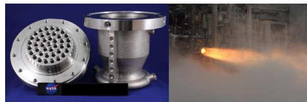
Figure 13. Additively Manufactured LOX/LCH 4 Pressure-Fed Main Engine
