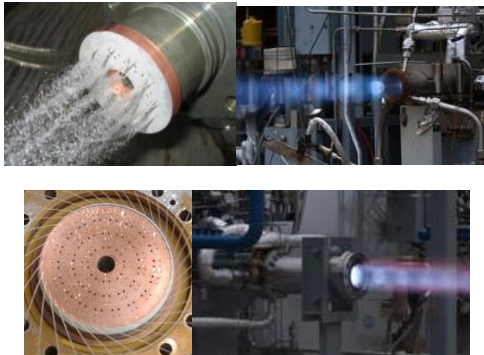
Figure 9. Impinging Injector Tests
