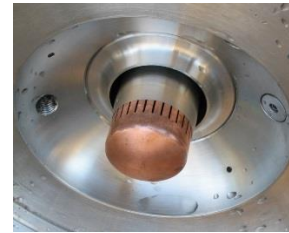
Figure 15. Northrop Grumman Throttling LOX/LH 2 Pintle injector
