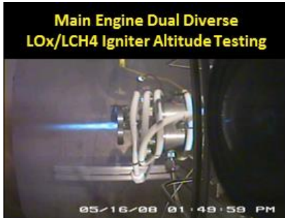
Figure 3. Dual, Diverse Ignition Torch (Firing)
