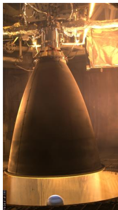
Figure 12. Aerojet 5500-lb f LOX/LCH 4 Main Engine Demonstration Testing
