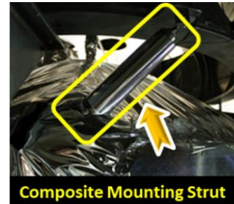
Figure 21. NASA's CPST Composite Strut Design, as installed.
