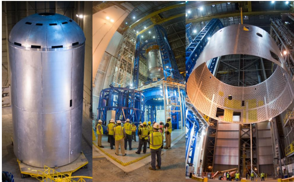
Figure IV: LH2, LOX, and engine section weld confidence articles at MAF.
