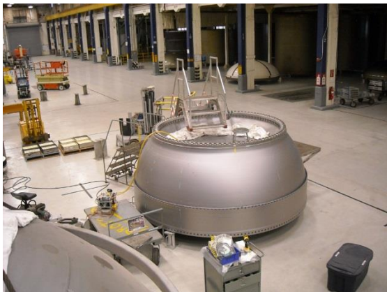
Figure 9: EM-1 LH booster aft dome refurbishment.
