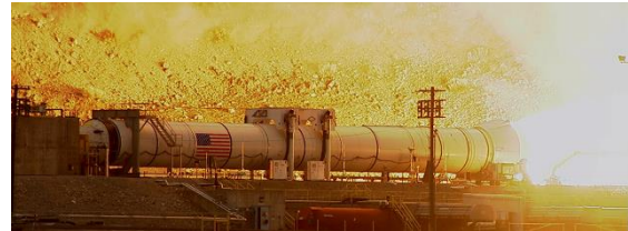
Figure 5: The QM-1 static test verified booster operations at 32 degrees Celsius (90 degrees Fahrenheit).
