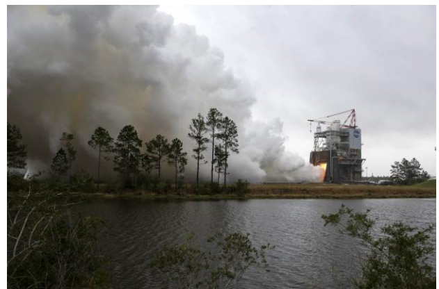
Figure 4. Testing of an EM-2 flight RS-25 engine at Stennis Space Center in Mississippi.
