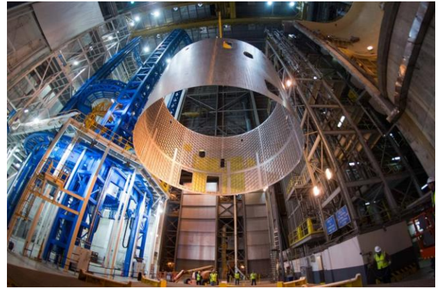
Figure 3. The core stage engine section weld confidence article at Michoud Assembly Facility.
