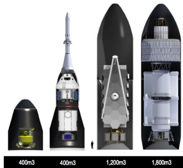
Figure 6. Fairing options for evolved configurations of Space Launch System.
