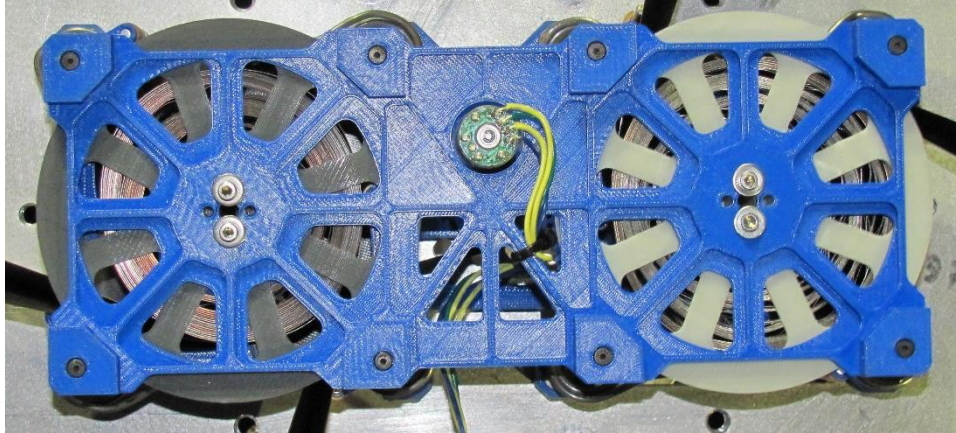
Figure 22. NeXolve (left) and AFRL (right) 4m TRAC booms spooled prior to first deployment
