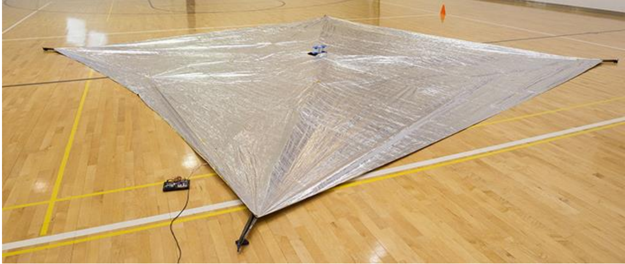
Figure 23. Deployed Solar Sail After Second Deployment
