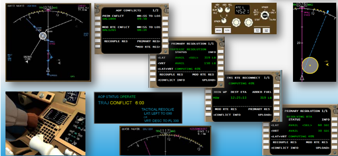
Figure 356 – Aircraft Automation Technologies for AFR
