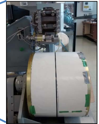
Commercial prepregger used to fabricate CNT yarn prepreg
