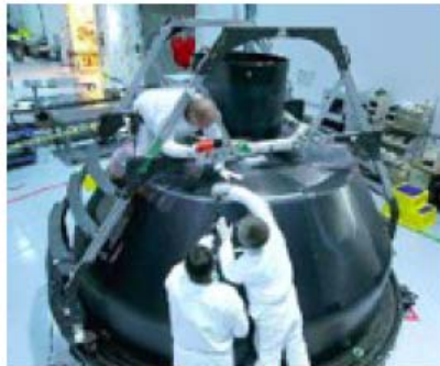
Future Composite Space Vehicles (NASA's Composite Crew Module)
