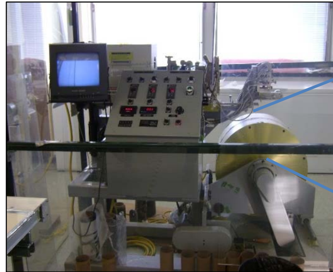
Commercial prepregger used to fabricate CNT yarn prepreg
