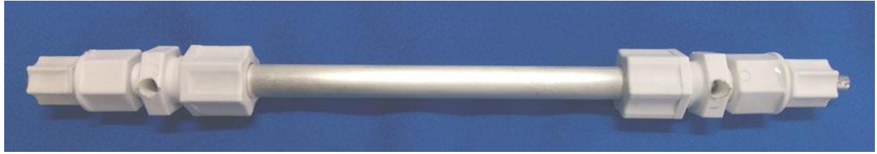
Figure 13. Membraneless tubular silver ion biocide cell
