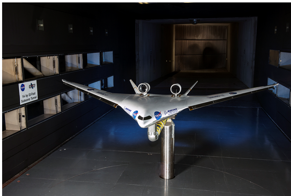
Figure 3: HWB model (flow-through nacelle configuration) installed in the NASA LaRC 14- by 22-foot Subsonic Wind Tunnel.
