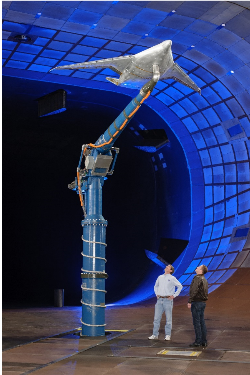
Figure 4: HWB FTN configuration installed in the NFAC 40- by 80-foot test section.
