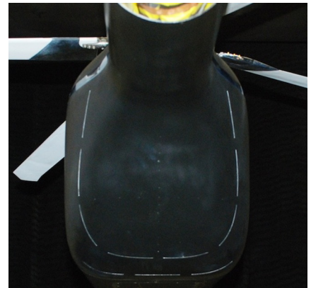
(f) Rear view of the model highlighting the actuator layout.
