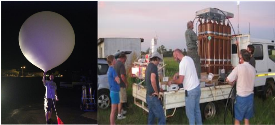
(Left). Medium balloon launch with sondes to measure aerosol backscatter . (Right) Preparation of the Optical Particle Counter flight under a large balloon.
