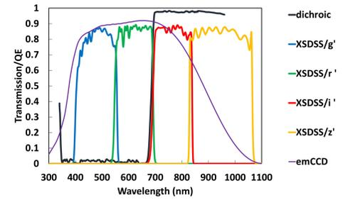
Detector QE/SDSS Filter Transmission
