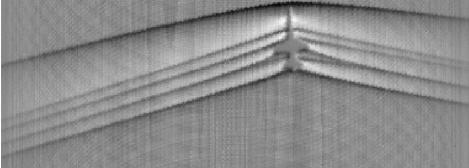
Using 10 subpixels per real pixel increases acuity, Mach lines in the plume can now be seen
