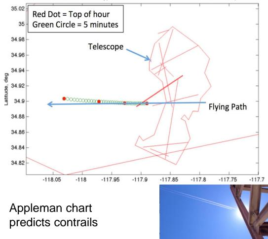
Ground to Air Schlieren Aircraft Waypoints for 09/06/2012 01:00PM to 04:00PM, Z=39K, Hp=37.173K
