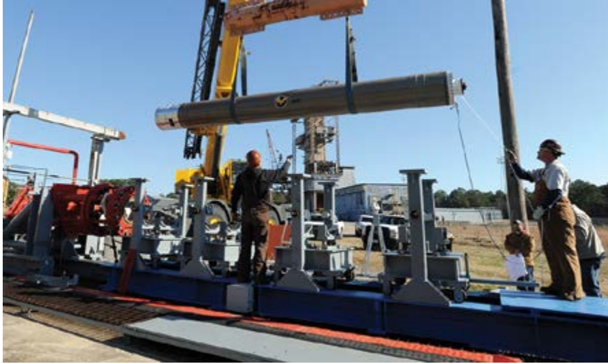
Motor loaded into test stand.
