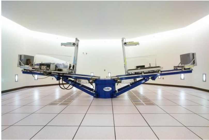
Figure 5. The tilted configuration of the centrifuge used in the NASA AG study. The centrifuge can accommodate 2 subjects in a HDT posture. A subject can be seen on the left of the two platforms. Photo courtesy of NASA/Wyle and obtained at the Red Orbit website at http://www.redorbit.com/news/space/147287/nasa_gives_artificial_gravity_a_spin/
