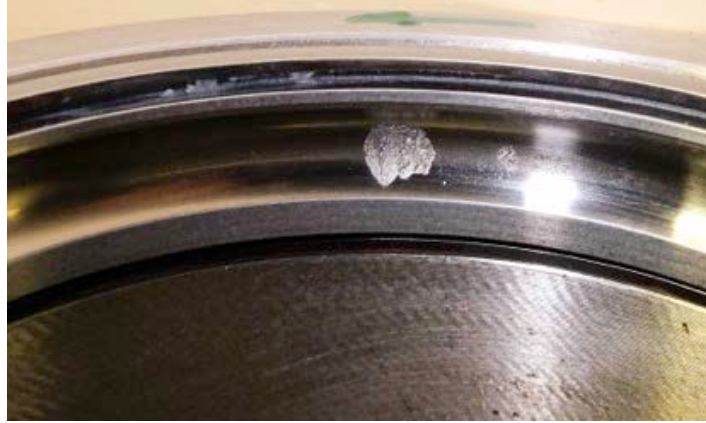
Figure 10. Raceway pit developed during shimmed bearing test after 157 hr of run-time
