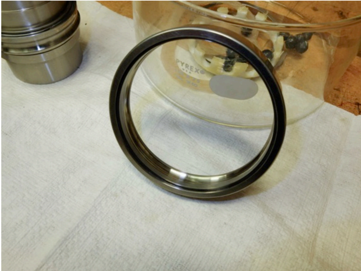
Figure 13. Photograph of the test bearing during an interim inspection at 1075 hr. Overall condition of the bearing races, balls and retainer was unchanged from beginning of test. The grease consistency and color was also unchanged
