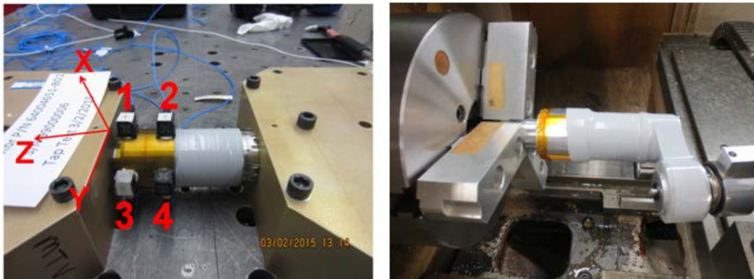
Figure 3. Left: Tap Test Set up. Right: SFT wrap set up.
