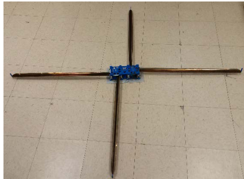
Figure 10. Boom Deployer Prototype with flight-like TRAC booms
