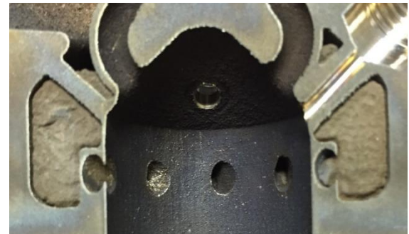
Entrapped compacted powder.
