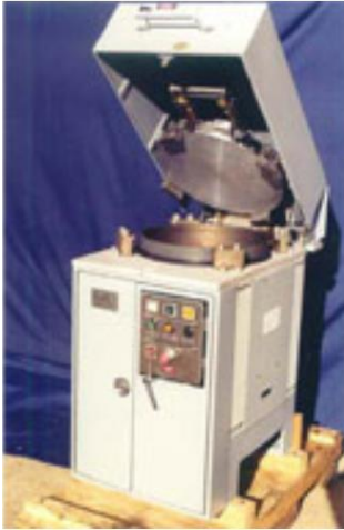
Figure 2. Compress Melt Unit – commercial system similar to one used by the Navy in 2003
