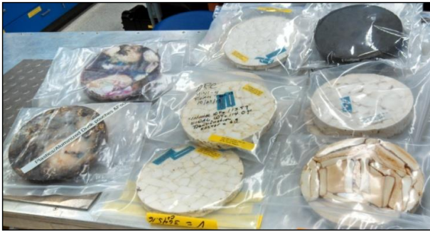
Figure 6. Gen1 Tiles. General trash on left, ISS packing foams in middle, Bosch carbon on upper right.
