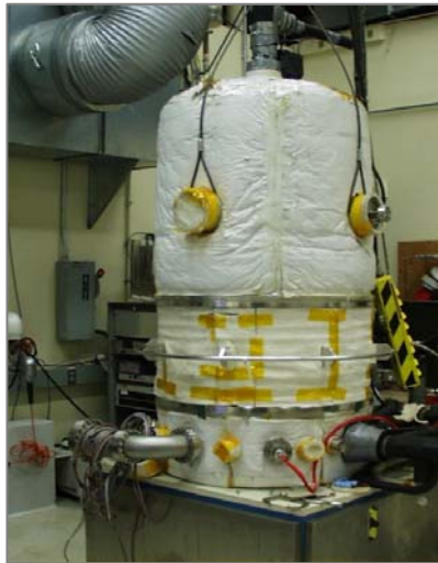
Figure 4. Dynavac Chamber with Shroud Extension Installed
