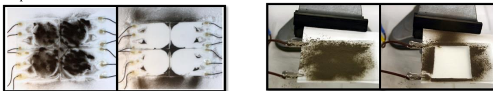
Figure 3. Demonstration of EDS feasibility on Optical surfaces (Left) and Glasses Surfaces (Right) 5 . These pictures show the before and after EDS activation states of various rigid surfaces. The surfaces are able to repel dust when EDS is activated.
