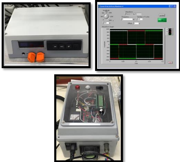
Figure 5. (Top Left) Three phase power supply. (Top Right) Multi-phase waveform timing diagram. (Bottom) Two Phase power supply.
