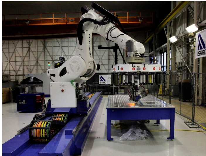
Figure 1. Simplified diagram showing the operating principles of Automated Fiber Placement (AFP) systems. In some designs the AFP head will remain stationary while the substrate translates and rotates on a spindle, such as during the construction of barrel fuselage sections.
