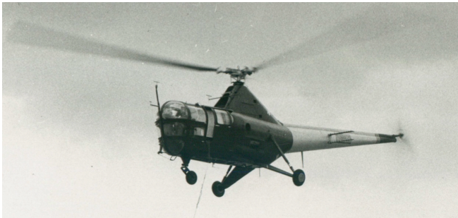
Figure 7. HO3S-1 with Langley developed horizontal tail.
