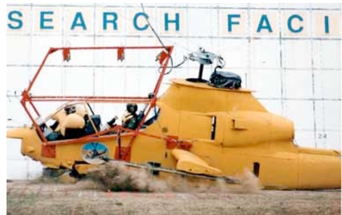
Figure 20. Crash test of AH-1S helicopter with CABS crew restraint systems.
