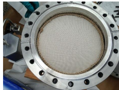
Figure 7: DPF test data: (a) plot of pressure drop, (b) images of the inlet and (c) outlet faces of the ceramic filter post-testing.
