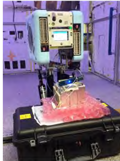
Electrical integration test • R2P1 on pink bubble wrap • Blue LED is RF indicator
