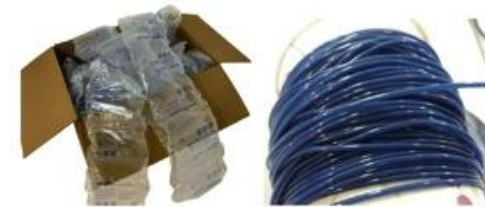
Figure 9. Polyethylene Packaging Material Before and After Processing with the Reultrafin Prototype Common Use Materials for 3D Printing & Packaging
