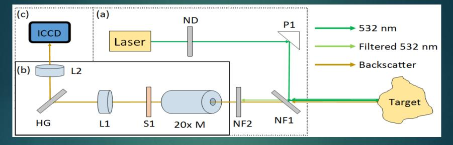
Block diagram of proposed system using a laser, neutral density filter (ND), a 45° mirror (P1), notch filters (NF1, NF2), A 20x magnification microscope objective (20x M), a slit (S1), achromatic lenses (L1, L2) a volume phase holographic grating (HG), and a mini ICCD camera.
