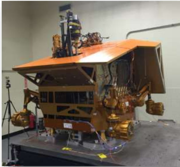
TVAC chamber X/Y-axes testing of RP15 rover
