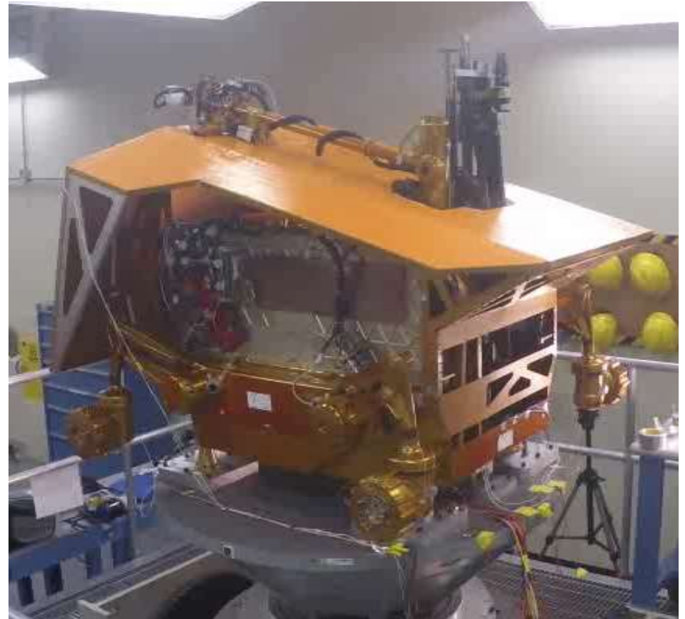
TVAC chamber Z-axis testing of RP15 rover
