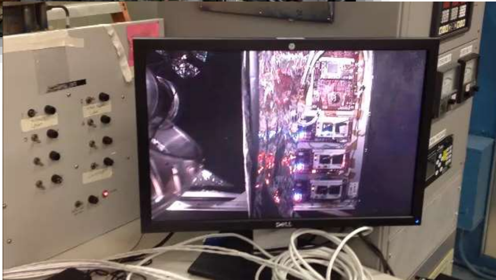
RP15 wheels & steering assemblies undergoing TVAC test
