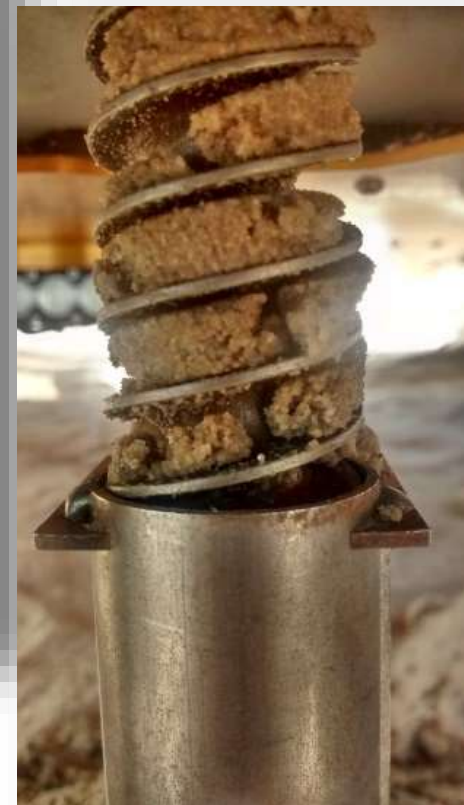
Sand Captured in Drill Brush Housing & Flutes
