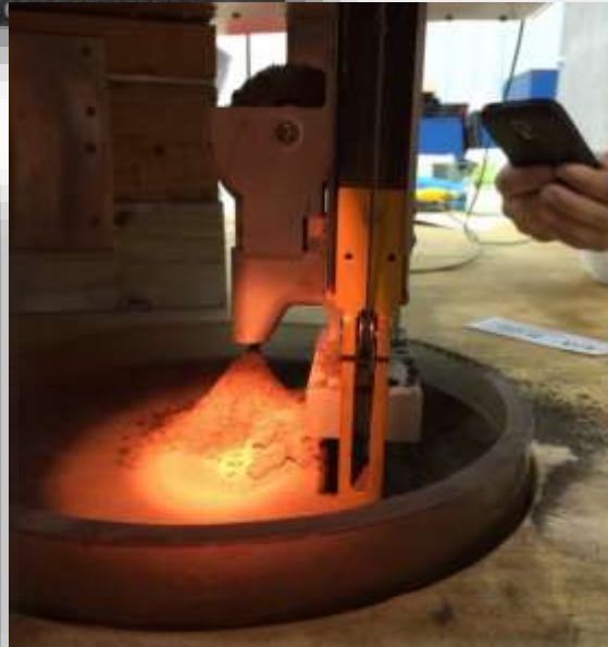
RP15 Rover-hosted Drill testing in doped simulant tube at NASA-JSC
