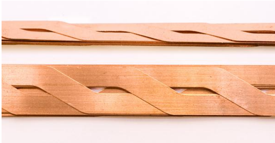
Figure 5: 15-strand HTS Roebel cable [7]
