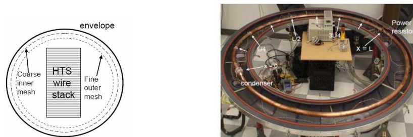
Figure 8: Cross-section of heat pipe (left) and cryogenic heatpipe (copper casing) in open toroidal vacuum chamber (right)
