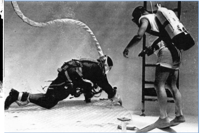
UPI Telephoto SPACE AIRLOCK — A model of an airlock, designed by McDonnell Company in St. Louis, to allow astronauts to transfer from spacecraft into an orbiting station, has been built for underwater training of the Apollo astronauts. Holes in the model will allow it to sink to the bottom of a large water tank where the astronauts will get a simulation of weightlessness while working the airlock.
