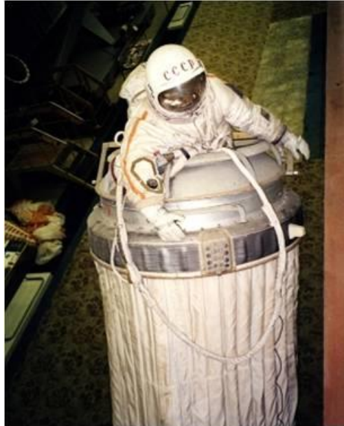
Fig. 2.4 (left) The Inflatable Airlock That Made The EVA Possible
