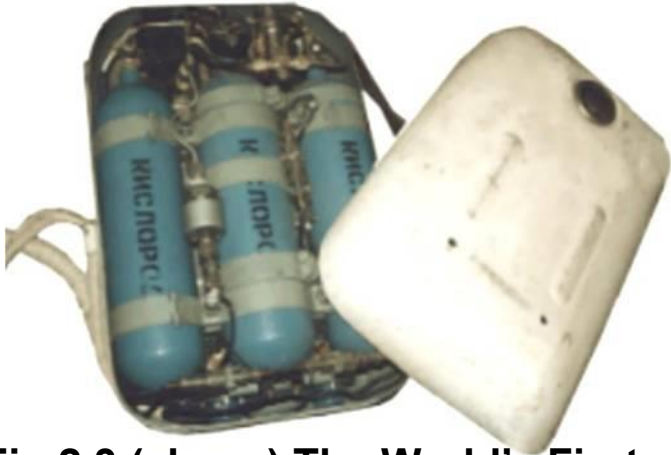
Fig 2.3 (above) The World's First EVA Life Support System
