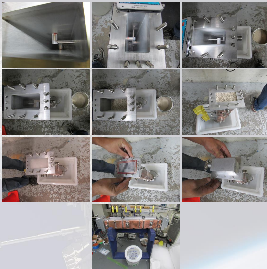
Figure 1. Loading of the WR340 rectangular waveguide based sorbent bed. Top to Bottom: (1 st Row, Left-) Empty bed; (1 st Row, Middle-) bed with quartz wool at bottom; (1 st Row, Right-) First layer of 13x added; (2 nd Row, Left-) Second layer added; (2 nd Row, Middle-) Third layer added; (2 nd Row, Right-) Final layer of 13x added; (3 rd Row, Left-) Top layer of quartz wool added; (3 rd Row, Middle-) Perforated plate added; (3 rd Row, Right-) Gas inlet/distributor end piece added; (4 th Row) Fully assembled bed.
