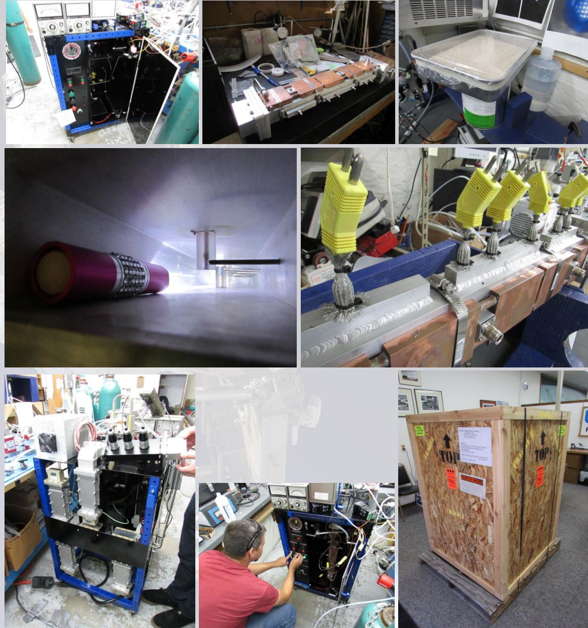
Figure 3. Preparation of the MRSHP prototype for delivery. Left to Right: (Upper Photos) Refurbishment- empty HGE, new cables w/ disassembled bed, media removed and saved; (Middle Photos) Reassembly- quartz sleeves affixed inside bed and shielding placed on thermocouple probes; (Lower Photos) Tuning, labeling, photos and shipping.
