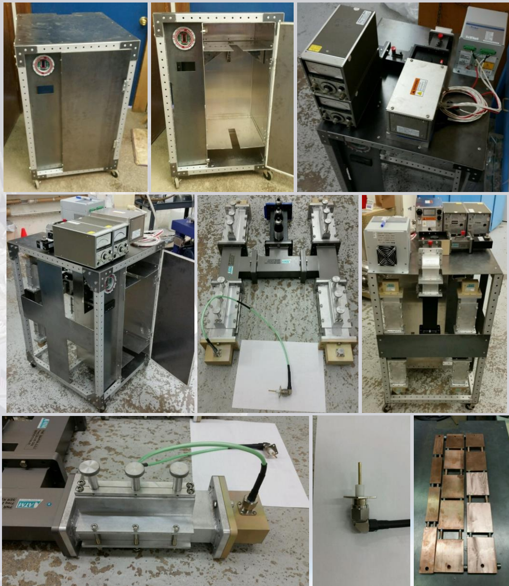
Figure 1. MRSHP prototype assembly. (Top Left-) Empty rack with door closed; (Top Center-) Empty rack with door open; (Top Right-) Rack with microwave hardware on top; (Middle Left-) Rack with waveguide H-mount; (Middle Center-) Waveguide H-assembly; (Middle Right-) Rack with waveguide H-assembly mounted; (Bottom Left-) Custom tuner, coax transition, coaxial cable and antenna; (Bottom Center-) Coaxial panel mount antenna; (Bottom Right-) Copper cooling plate assemblies.
