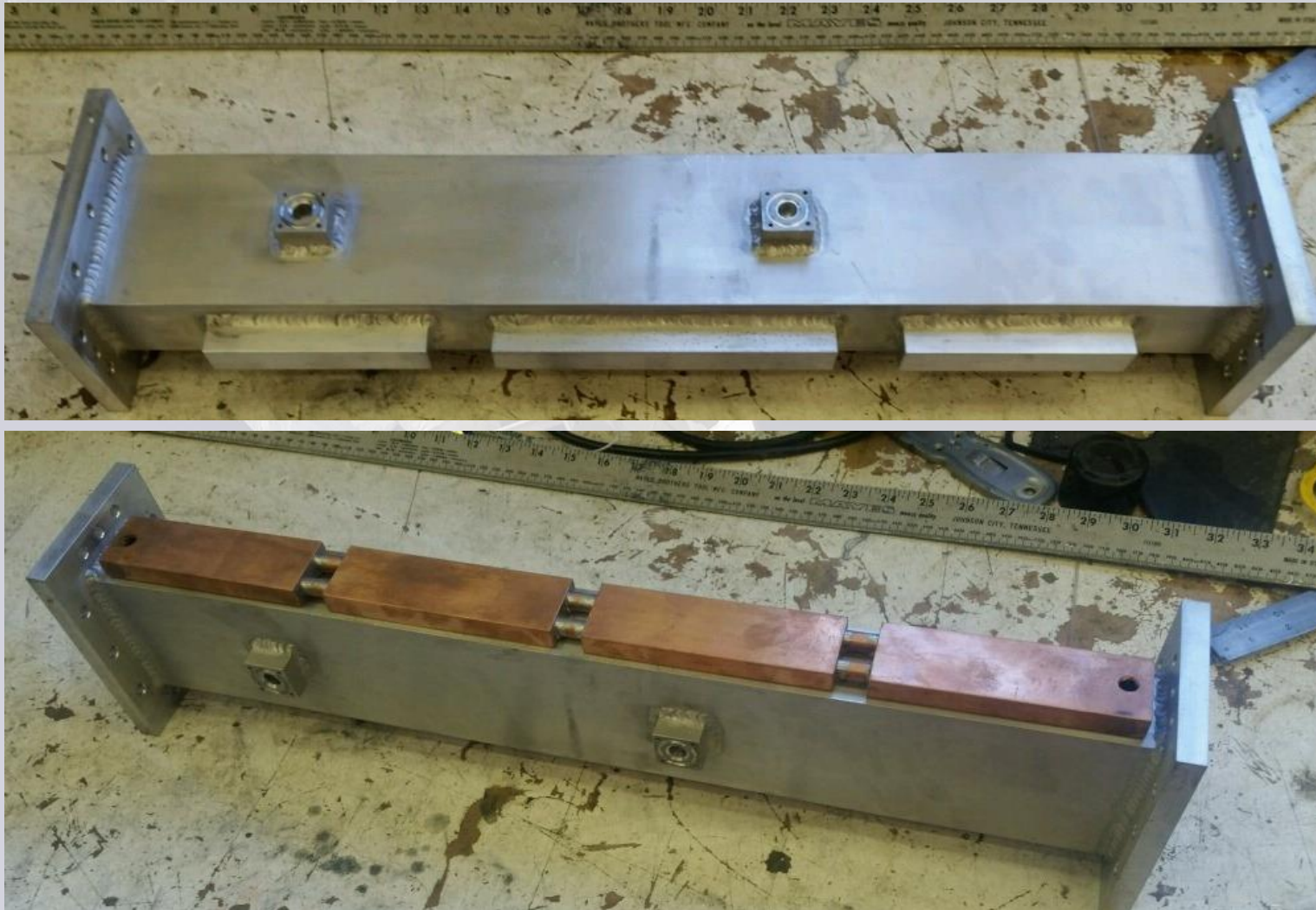
Figure 2. MRSHP waveguide bed. (Upper-) WR340 Bed; (Lower-) Bed and narrow side cooling plates.
