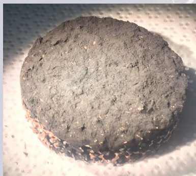
Fe-coated copper from [bmpyrr][SO 4 ]
