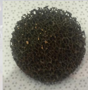
Fe-coated copper from [emim][SO 4 ]
