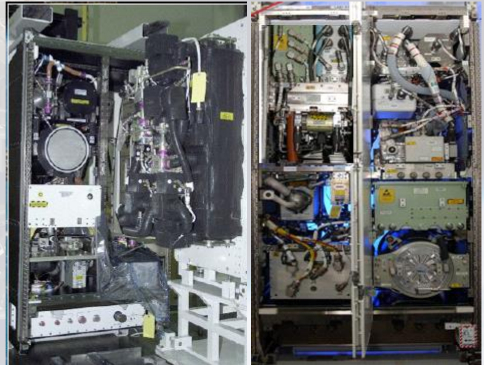
ISS Atmosphere Revitalization Rack (left) and Oxygen Generation System Rack (right)
