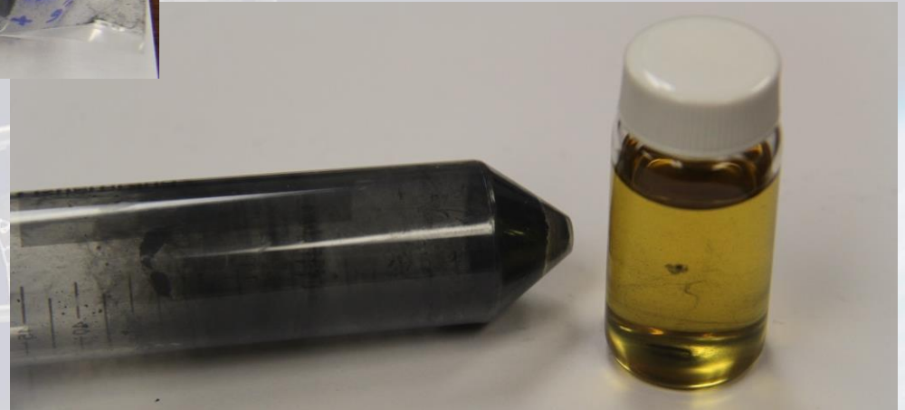
Carbon residue following IL extraction of Fe (left) and IL containing Fe with small quantities of residual carbon (right).
