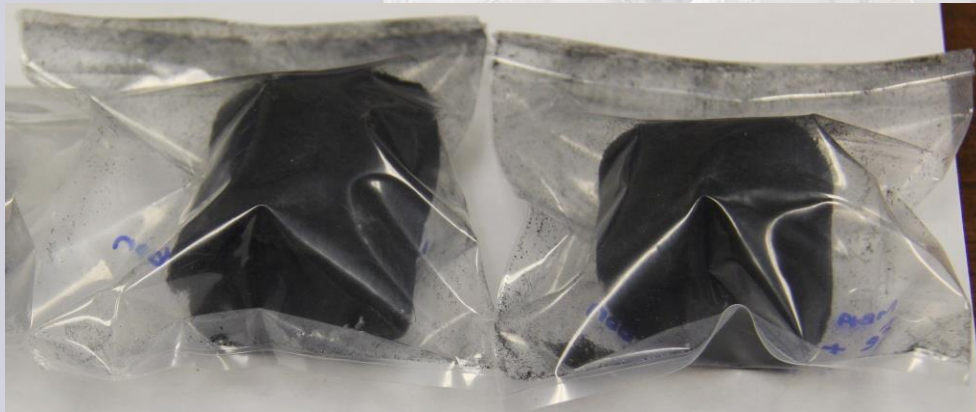
Fe wool coated in carbon during previous Bosch catalyst development testing.
