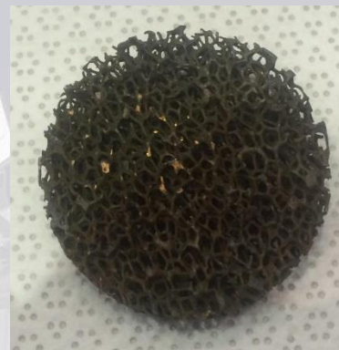
Fe-coated copper from [emim][SO 4 ]
