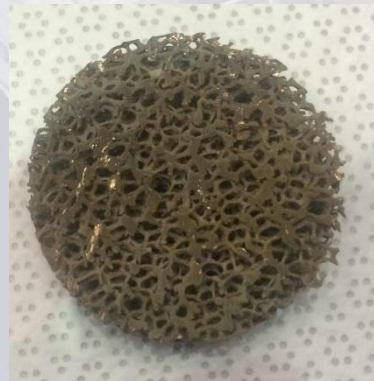
Fe-coated copper from [bmpyrr][SO 4 ]
