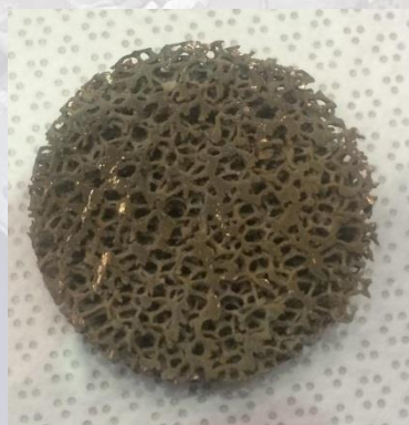
Fe-coated copper from [bmpyrr][SO 4 ]
