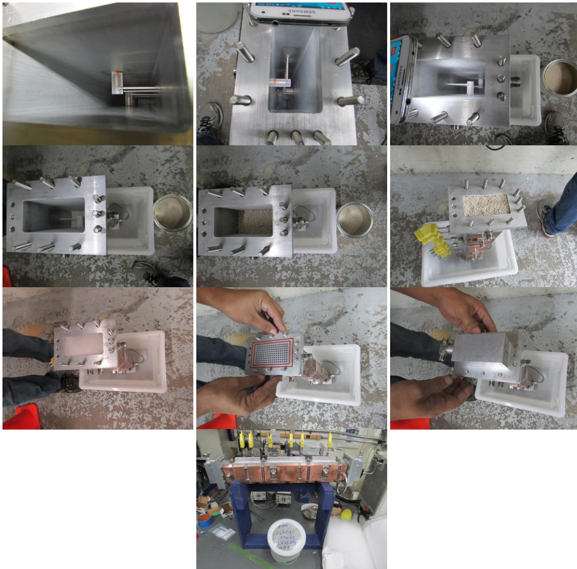
Figure A2. Loading of the WR340 rectangular waveguide based sorbent bed. Top to Bottom: (1 st Row, Left-) Empty bed; (1 st Row, Middle-) bed with quartz wool at bottom; (1 st Row, Right-) First layer of 13x added; (2 nd Row, Left-) Second layer added; (2 nd Row, Middle-) Third layer added; (2 nd Row, Right-) Final layer of 13x added; (3 rd Row, Left-) Top layer of quartz wool added; (3 rd Row, Middle-) Perforated plate added; (3 rd Row, Right-) Gas inlet/distributor end piece added; (4 th Row) Fully assembled bed. 2.2 L of Grace-Davison molecular sieve 13x media, received from Marshall Space Flight Center, was used to fill the waveguide based bed.
