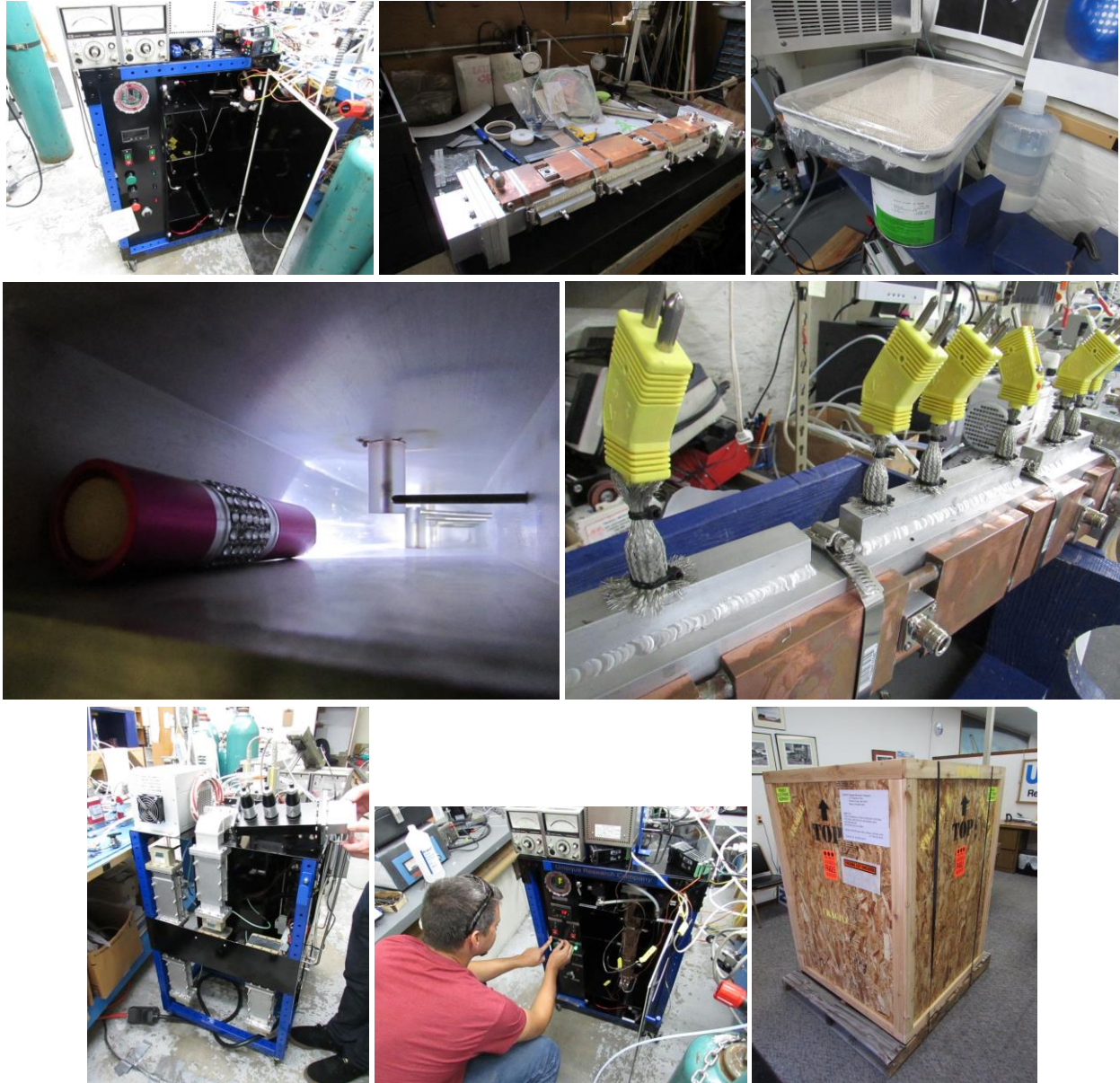
Figure A3. Preparation of the MRSHP prototype for delivery. Left to Right: (Upper Photos) Refurbishment-empty HGE, new cables w/ disassembled bed, media removed and saved; (Middle Photos) Reassembly- quartz sleeves affixed inside bed and shielding placed on thermocouple probes; (Lower Photos) Tuning, labeling, and preparation for shipping.
