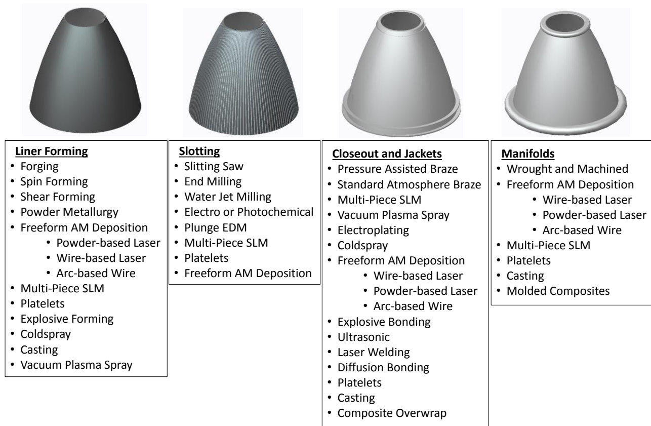
Figure 2. Various fabrication processes for channel wall nozzle liners, slotting, closeout and manifolds.
