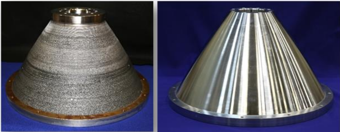
Figure 3. Blown powder deposition freeform liners fabricated, 24 inch diameter.
