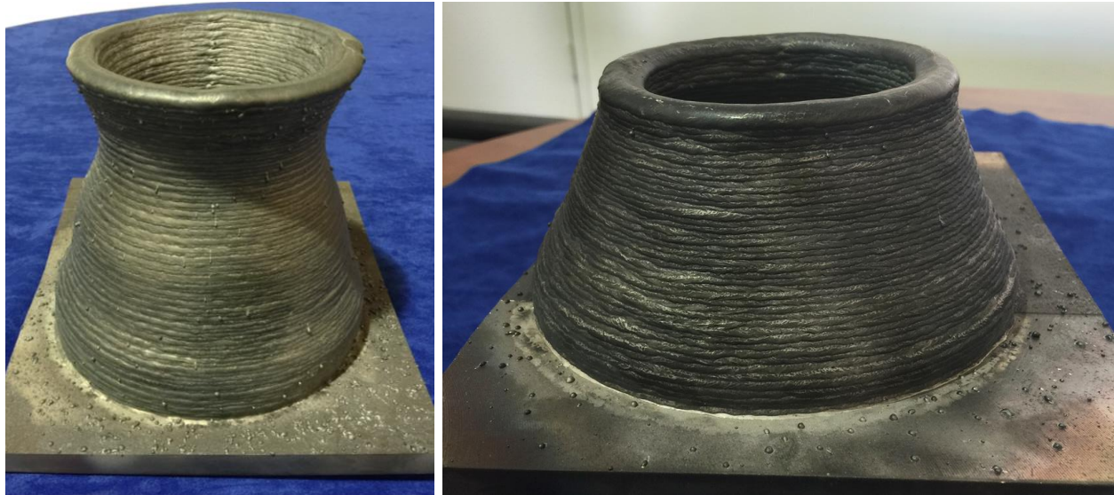
Figure 5. Example of Inconel 625 liners using arc-based freeform deposition, MDDM.
