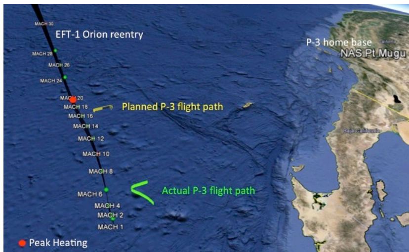
Figure 6-4. EFT-1 Capsule Reentry Track and Flight Path of the BH-300 Observation Aircraft (Planned, Yellow; Actual, Green)
